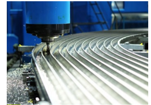
Serial production of 35 radial plates for ITER
